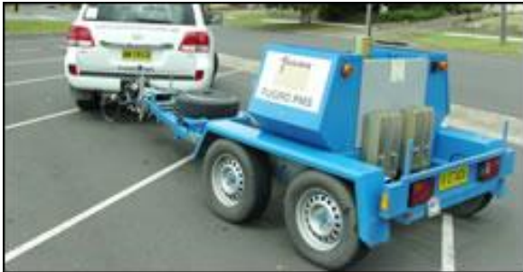
Figure 11.3 Falling Weight Deflectometer Unit 7
